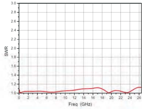
71802 DC block insertion loss & SWR vs. frequency
